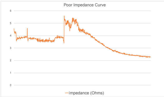
Example of poor impedance curve – more erratic & > 4 ohms during the infusion
